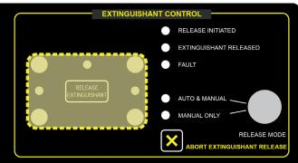
A time delay of 15 seconds will pass before the discharge signal is sent.
