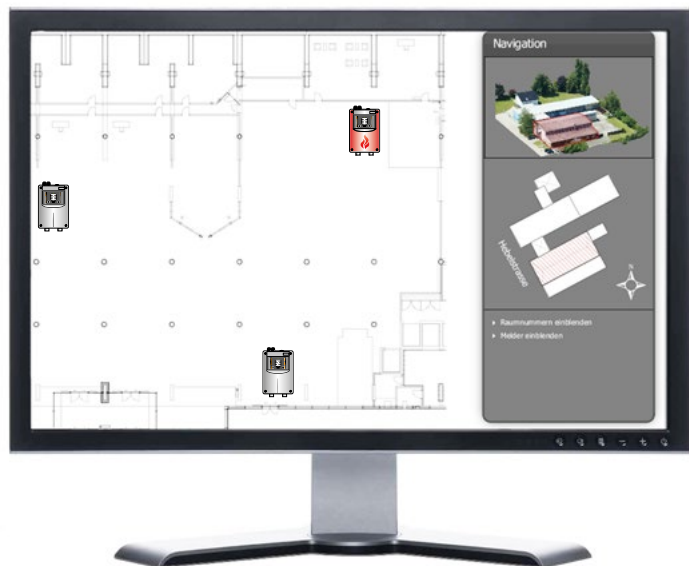
On-screen overview in NetSoft: installation with three aspirating smoke detectors.
