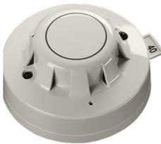
The **Discovery Marine Ionisation Smoke Detector** uses a low activity radioactive foil to detect fires by irradiating the air in the smoke chamber and causing a current flow. If smoke enters the chamber, the current flow is reduced leading to an alarm.
