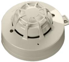
The **Discovery Marine Multi-sensor Detector** comprises optical smoke and thermistor temperature sensors which give both a combined signal as well as a separate heat signal for improved false alarm management.
